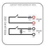
MSS-2##C-002: Series & Parallel 1k resistors on circuit A, Series 1k resistor on Circuit B. One instance shown at right:
