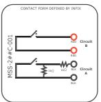
MSS-2##C-001: Series & Parallel 1k resistors on circuit A. One instance shown at right:
