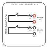
MSS-2##C-004: Series 1k resistor on Circuit A and on Circuit B. One instance shown at right:
