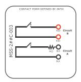
MSS-2##C-003: Series 1k resistor on Circuit A. One instance shown at right:
