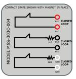
For End-Of-Line Resistor Custom Models Contact Magnasphere Corp.
