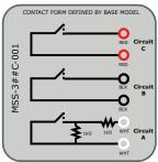
MSS-3##C-001: Series & Parallel 1k resistors on circuit A. One instance shown at right:
